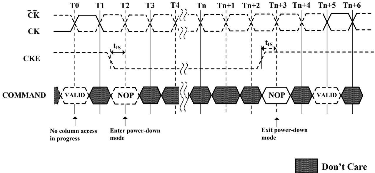
Figure 45. Clock Frequency Change in Precharge
