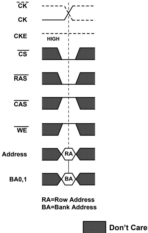
Figure 7. t<sub>RCD</sub> and t<sub>RRD</sub> Definition
