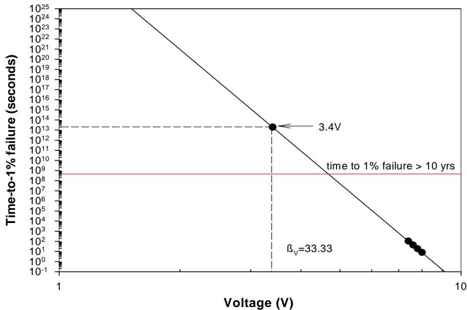
Figure 4: Time to 1% Failure as a Function of Stress Voltage (Thick Gate Oxide)
