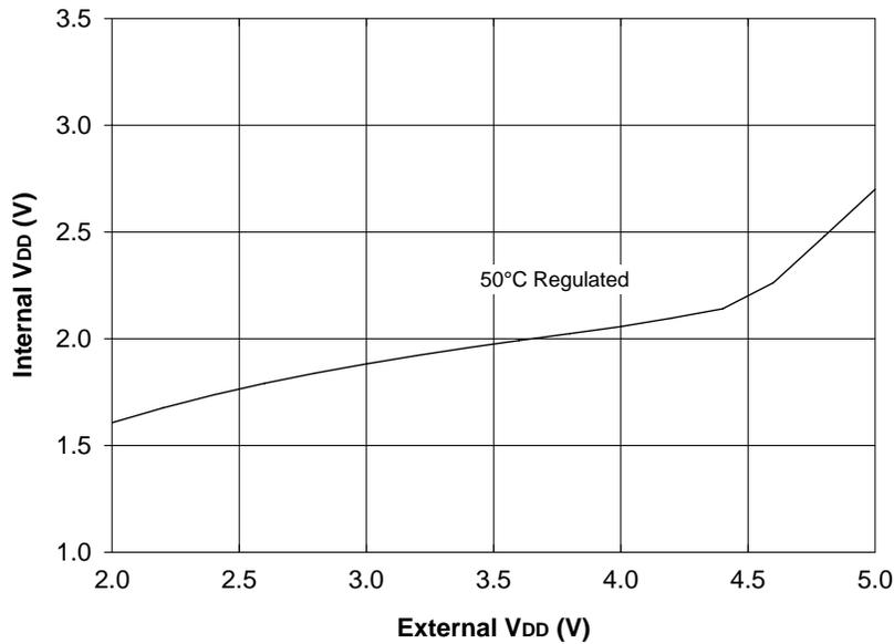
**Figure 1: Internal versus External VDD Levels for 3.3V device, 50°C**
