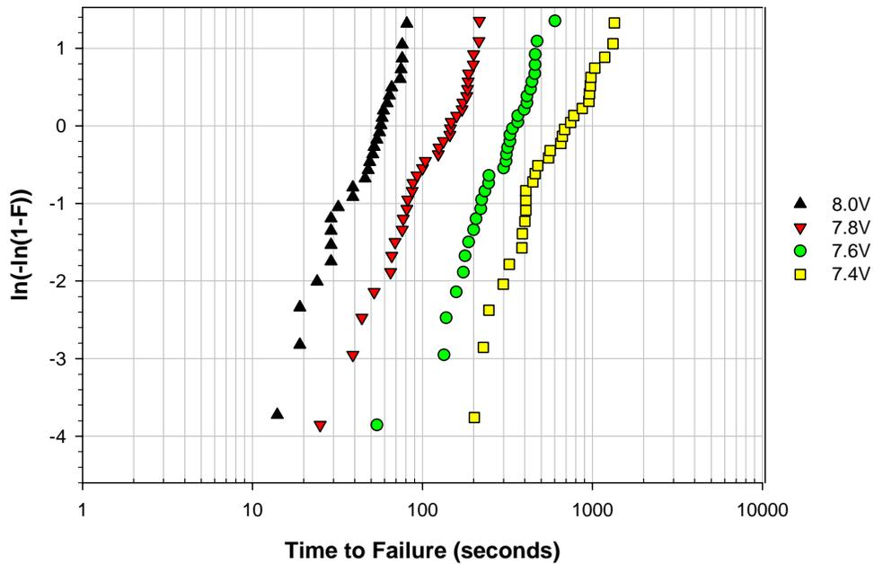
Figure 3: Weibull Distribution of Failure Times at Various Stress Levels (Thick Gate Oxide)
