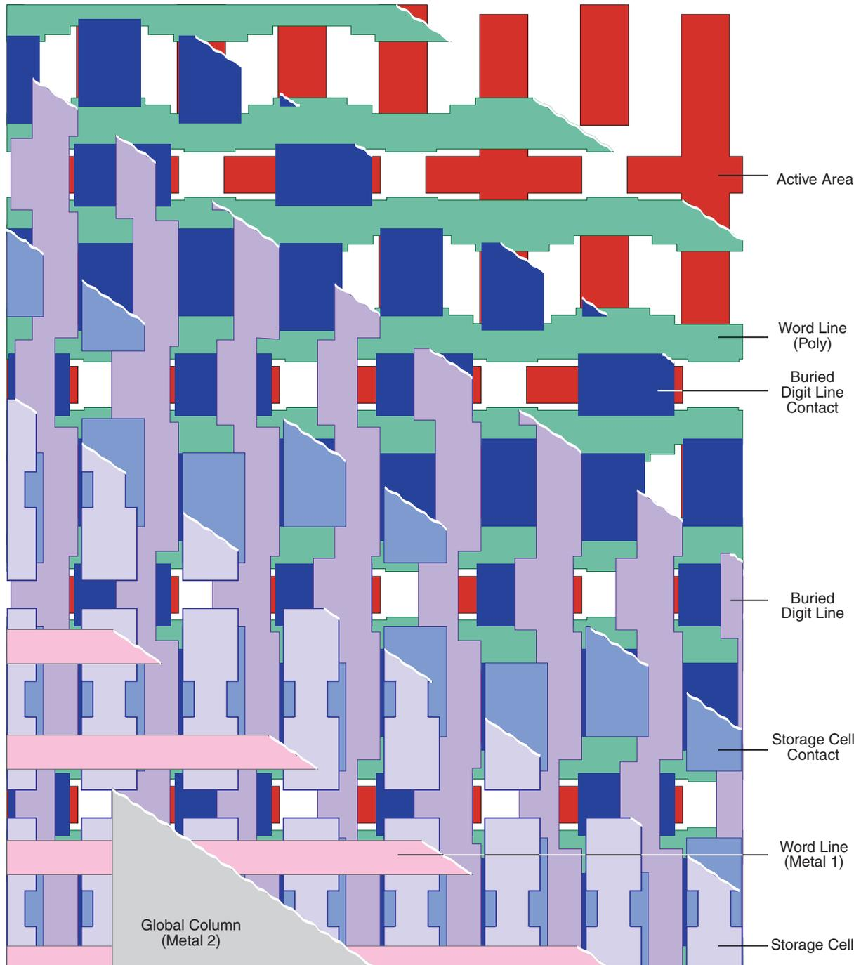
**Figure 22: Memory Cell Definition — Top-Down View**
