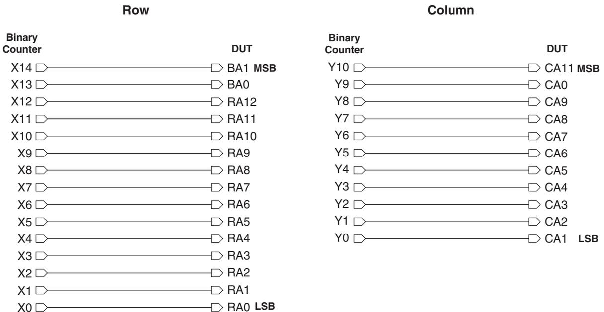
Figure 13: Address Topological Diagram — 64 Meg x 8
