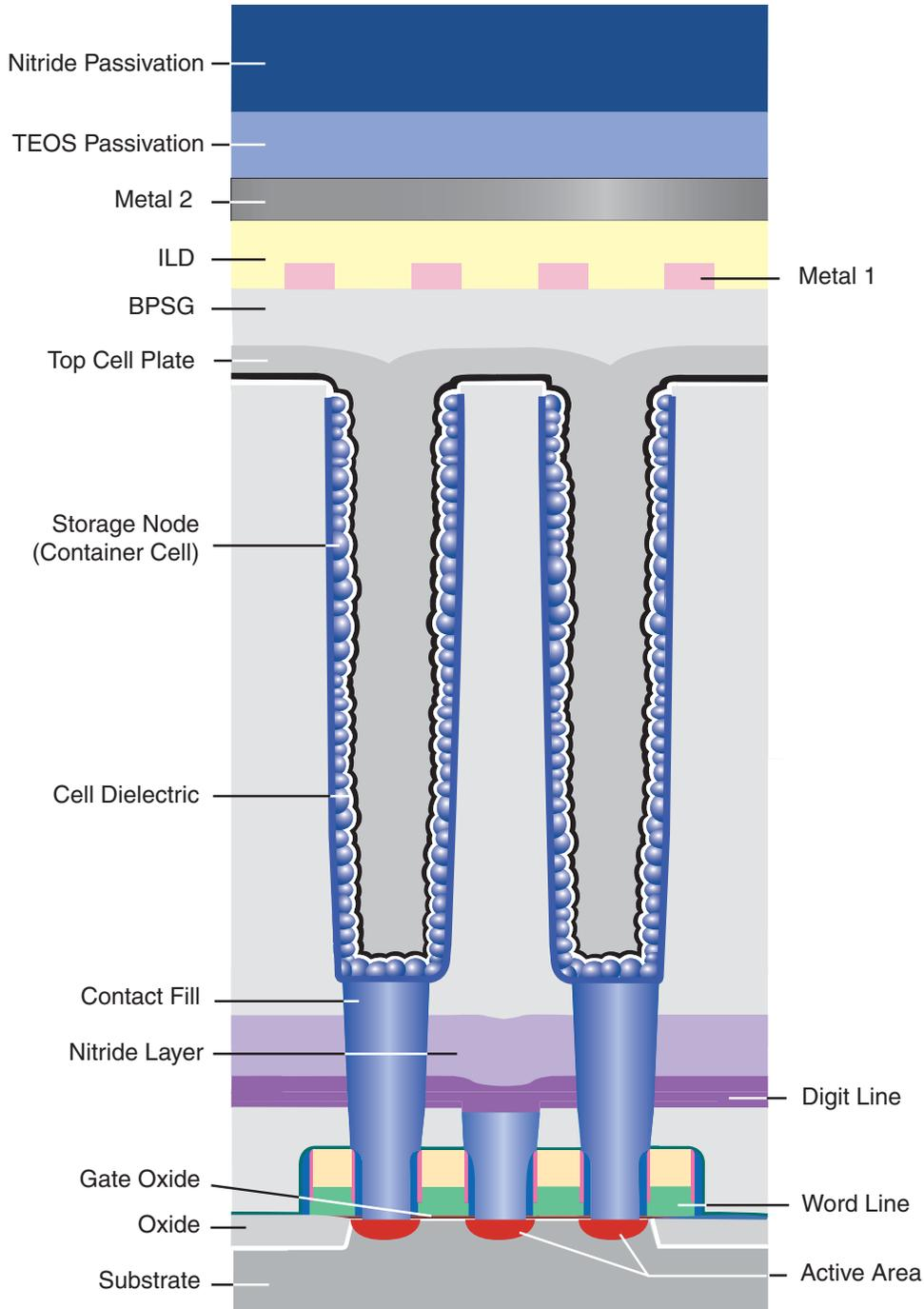
**Figure 23: Memory Cell Definition — Cross Section View**
