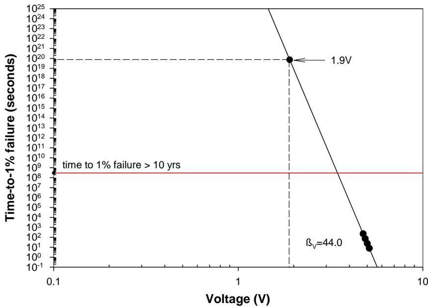
Figure 6: Time to 1% Failure as a Function of Stress Voltage (Thin Gate Oxide)
