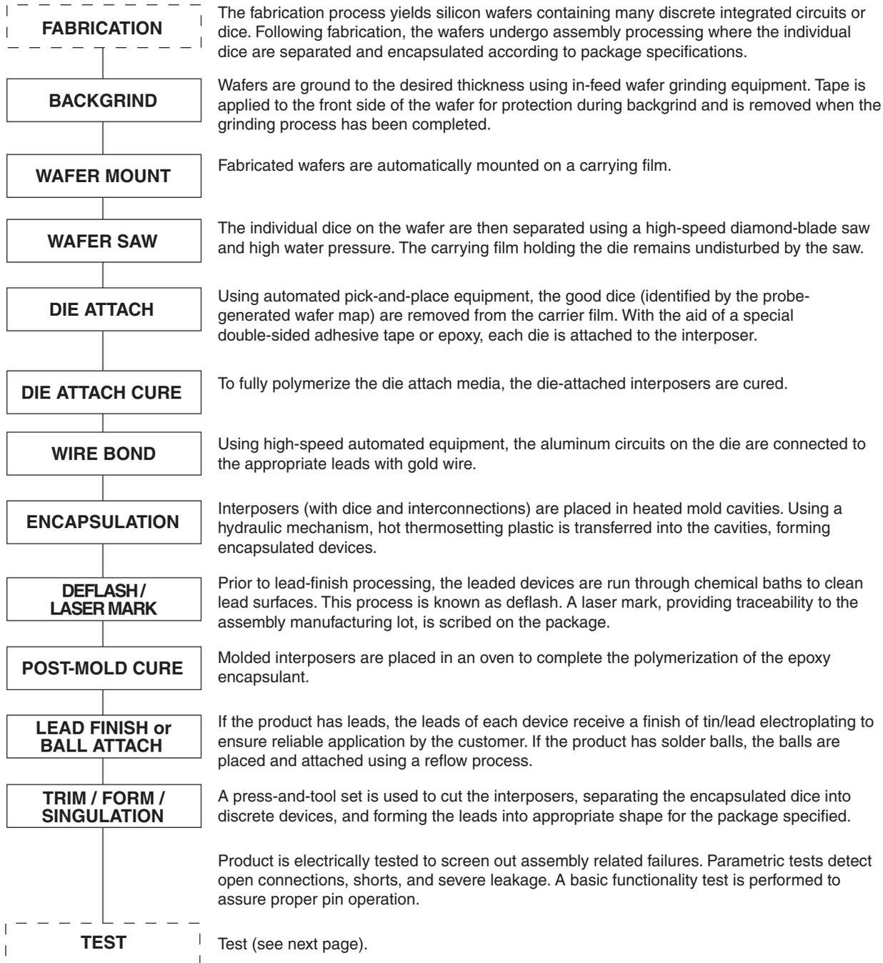
**Figure 26: Assembly Process Flow**
