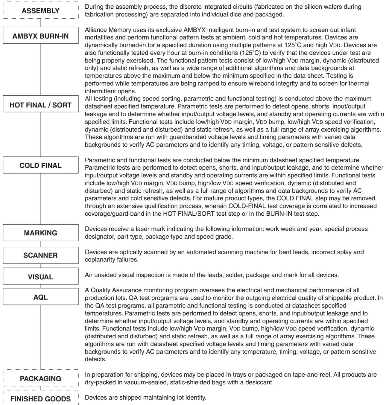
**Figure 27: Test Process Flow — Packaged Parts**
