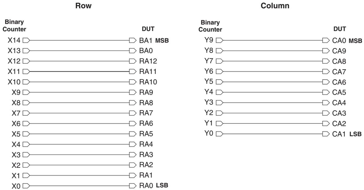
**Figure 14: Address Topological Diagram — 32 Meg × 16**
