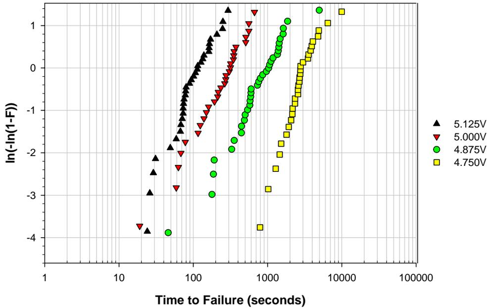
Figure 5: Weibull Distribution of Failure Times at Various Stress Levels (Thin Gate Oxide)
