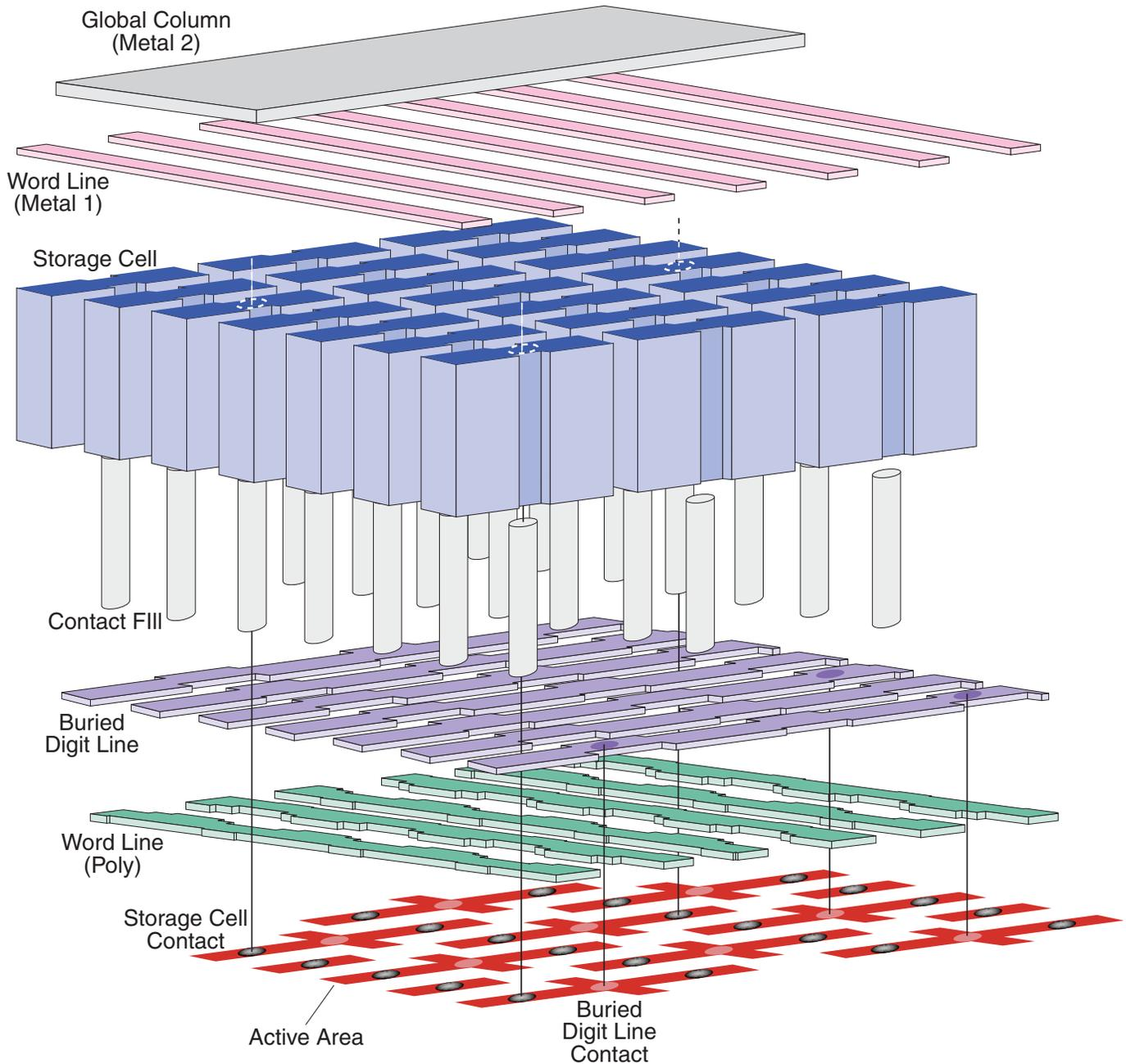
**Figure 21: Memory Cell Definition — Exploded View**
