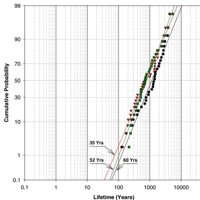
**Figure 7: Via Electromigration Log Normal Plot**
