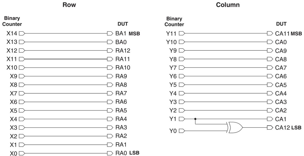
Figure 12: Address Topological Diagram — 128 Meg x 4
