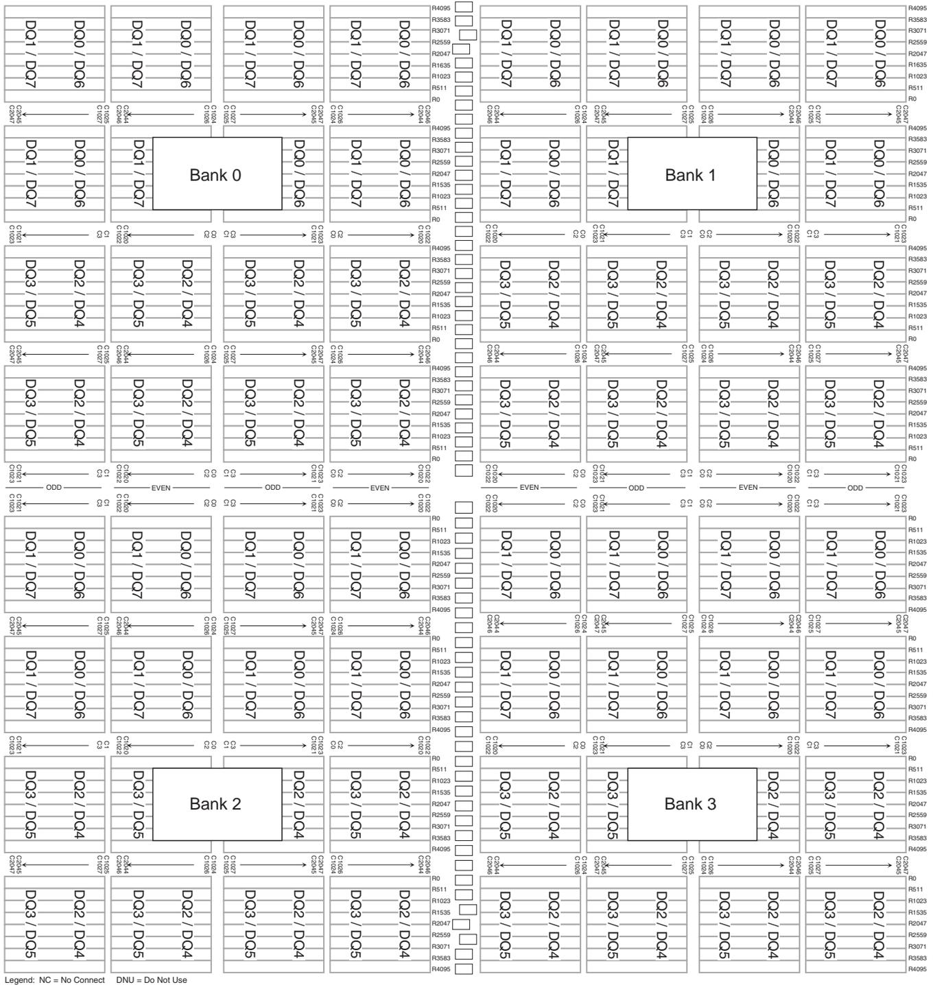
**Figure 10: Array Configuration — 64 Meg x 8**
