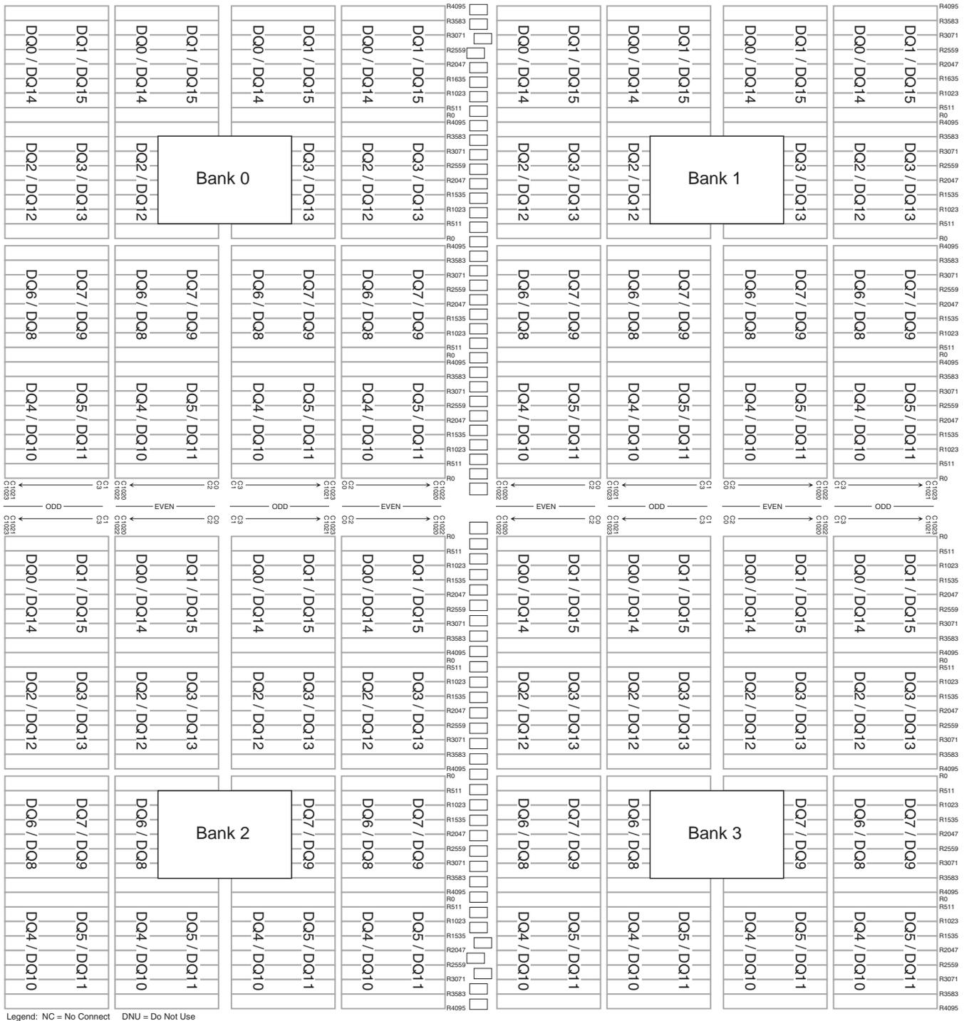
**Figure 11: Array Configuration — 32 Meg x 16**
